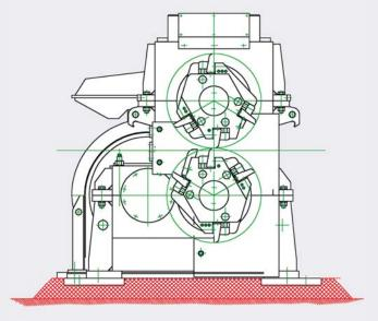
Shear start is initiated by pulse generator (billet head end). Cut according to chosen crop length. After cutting, the shear is stopped again. Crop end diverted into scrap disposal system.
