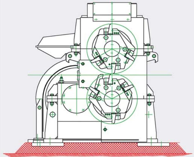
Shear start is initiated by pulse generator (billet head end). Cut according to chosen crop length. After cutting, the shear is stopped again. Crop end diverted into scrap disposal system.
