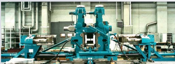
Universal mill stand in roll changing device, vertical rolls disassembled
